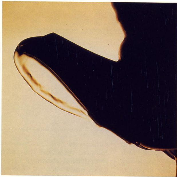
Figure 4. Pouring liquid from teapot demonstrates the "teapot effect." Detergent bottle shows lip designed to avoid "teapot effect"; design matches finite element predictions.
