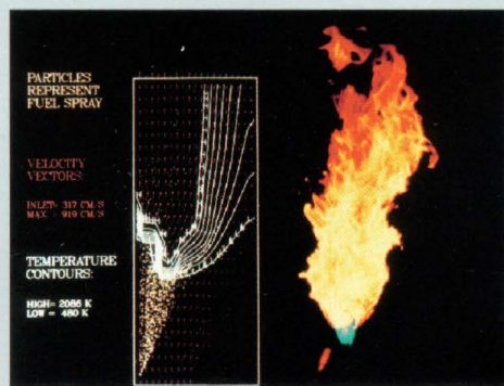
KIVA simulation (left) and experiment (right) of a continuous spray combustor.
