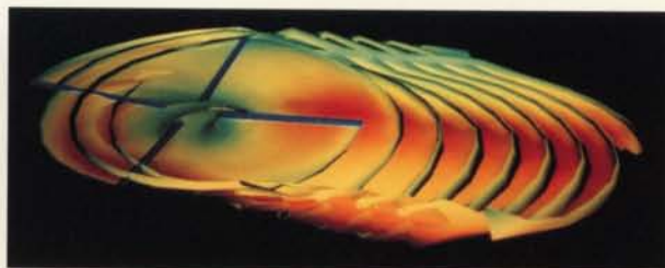
Right, three-dimensional view of the predicted vortex lattice wake structure modeling the complete wake surface of an H-34 helicopter rotor.
