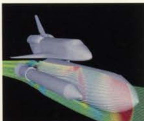
Left, airflow around ascending space shuttle. The image was generated using Cray Research's Multipurpose Graphic System, and includes a complete shuttle, tank, and solid rocket booster.
