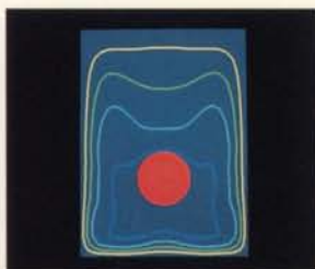
Left, temperature contours in canned food (meatball surrounded by liquid broth) undergoing sterilization. Modeling can improve process designs and reduce energy costs.
