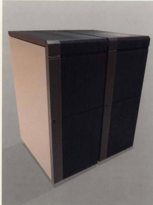
Two DE-60 disk cabinets, each containing up to eight DD-60 or DD-61 disk drives.
