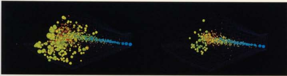
Fuel injection in a direct injection diesel engine during cold start.
