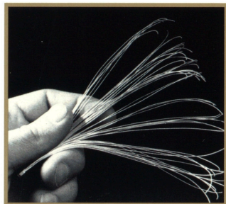
Above: The micro-coaxial cable used for inter-module communication.
